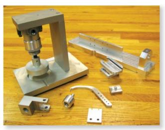
An overview of multiple parts milled on Roland MDX-540 during a two-week period at Cardiovascular Systems, Inc., a medical device company. Images courtesy Roland DGA and Cardiovascular Systems, Inc.
